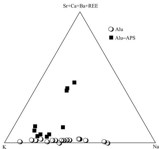
Fig. 5. D-position diagram of alunite (Alu) and alunite-APS s.s. (Alu-APS)
